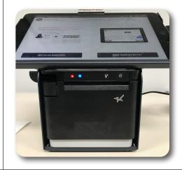
There will be a red light on the face of the printer when the printer tape starts running low.
